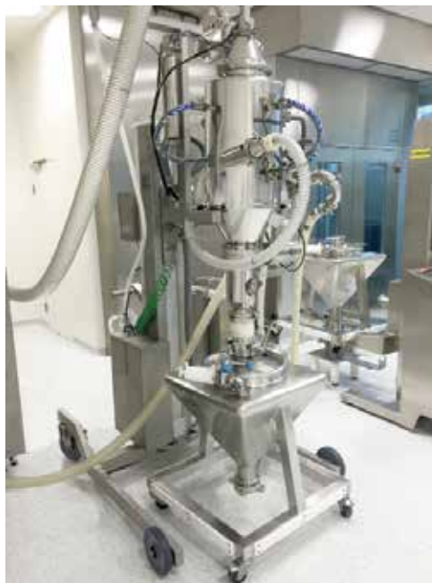
Photo 3: OEB 5 containment was verified in prepared clean room, with the vacuum conveyor mounted in a mobile frame and connected to an empty intermediate bulk container by a double-flap valve.
