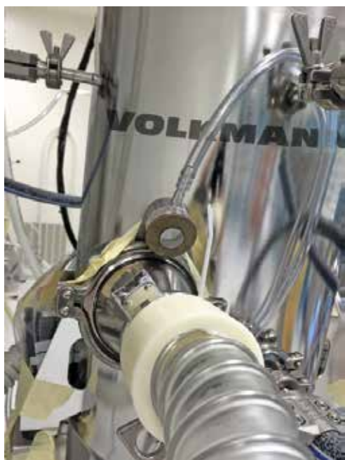
Photo 1: Lightweight sanitary hoses with molded cuffs provide simple connection to a vacuum receiver.
